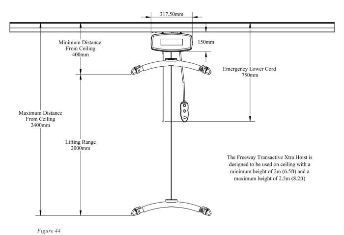
The diagram above (Figure 44) shows the relevant lifting ranges and dimensional sizes of the Hoist. The direction of travel can only be made within the boundaries of where the Hoist is in the track system.
