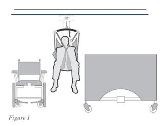
The Transactive Xtra Hoist is a Ceiling Track Hoist, and should only be used whilst on the Ceiling Track. It has the ability to raise up an individual from one location, such as a bed, move the individual along the track to another location and finally lower the individual, such as into a chair or a bath.
